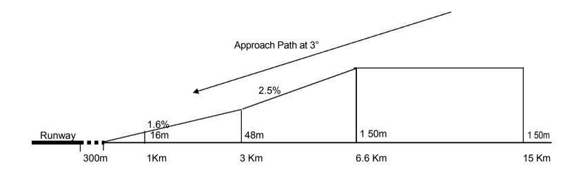
(Fig. 1: Allowable obstructions at various distances on  $\pm$  15° from the centerline of the runway)
